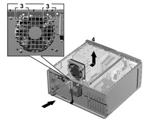
4. Disconnect the fan connector from the CHASSIS\_FAN socket on the system board.
